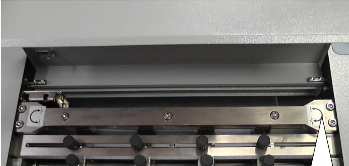
Find 4 screws on both side, turn the Allen screw according to the label beside to make the crease line deeper or light
