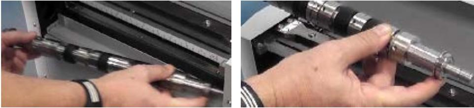
4. After all anvil is mounted again, install the shaft back, so to the clip.
